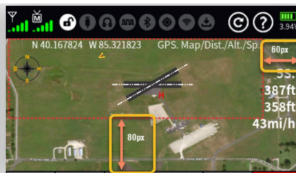
Measure the number of pixels from the bottom of the image (South Boundary) to the rectangle and do the same from the right (East Boundary).
